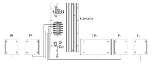
Fig. 6. Connections of the Subwoofer, the Center, the Front and the Surround Speakers
