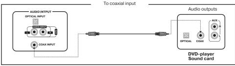
Fig. 7. Sound source installation diagram
