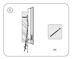
• To unmount your TV, release the security locks by pulling the tabs down (see Fig. ③). Lift your TV slightly and take the screws out of the holes.
