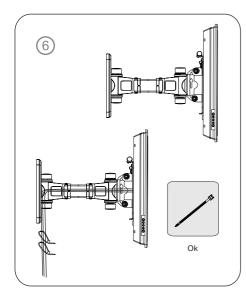
• To unmount your TV, release the security locks by pressing down on them (see Fig. ①). Lift your TV slightly and take the screws out of the holes.
